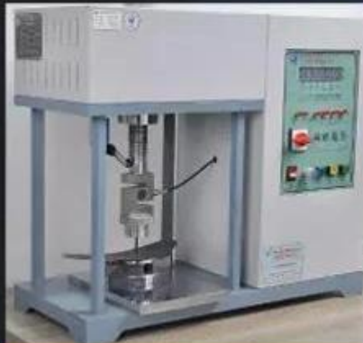
Midsole Test \geq 1200 Newtons
