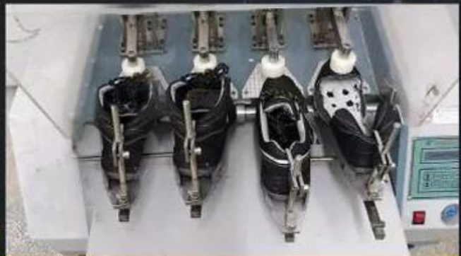
Flex Tester \geq 36,000 T
