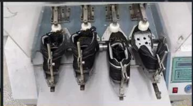
Flex Tester \geq 36,000T
