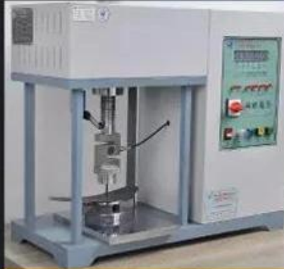
Midsole Test \geq 1200 Newtons
