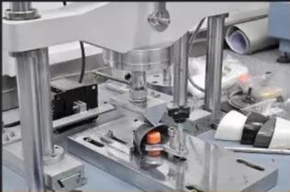
Toecap Test \geq 200 Joules
