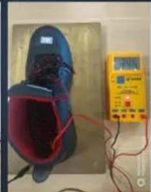
ESD Anti-Static Test
