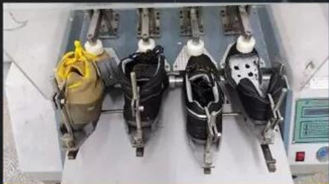
Flex Tester \geq 36,000 T
