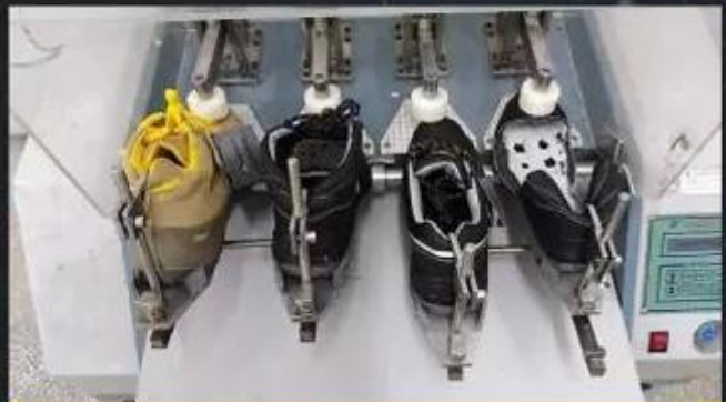
Flex Tester \geq 36,000 T
