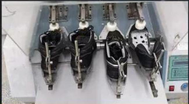
Flex Tester \geq 36,000 T
