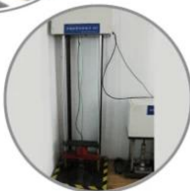
Impact Resistant Testing Machine
