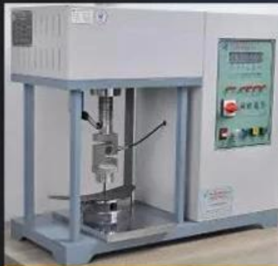
Midsole Test \geq 1200 Newtons
