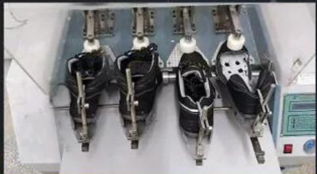
Flex Tester \geq 36,000 T
