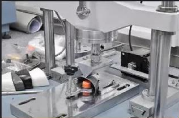
Toecap Test \geq 200 Joules
