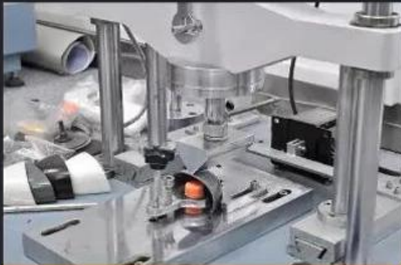
Toecap Test \geq 200 Joules
