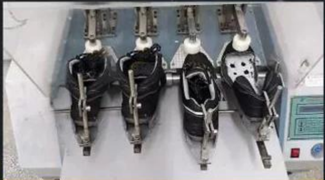
Flex Tester \geq 36,000 T
