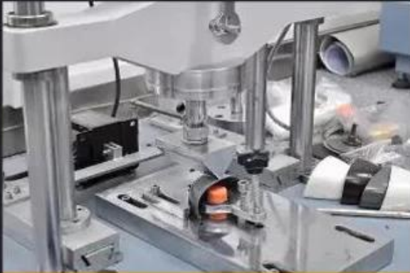
Toecap Test \geq 200 Joules
