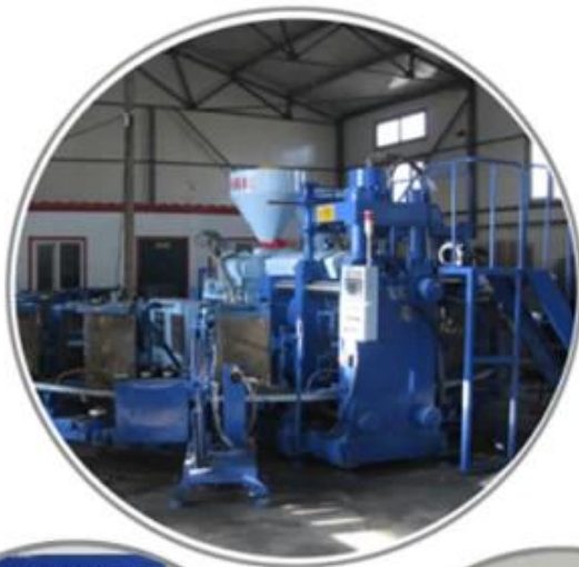
Automatic Injection Molding Machine
