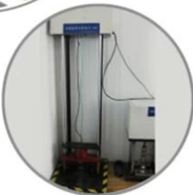
Impact Resistant Testing Machine
