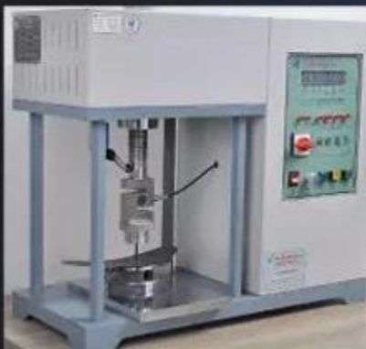
Midsole Test \geq 1200 Newtons
