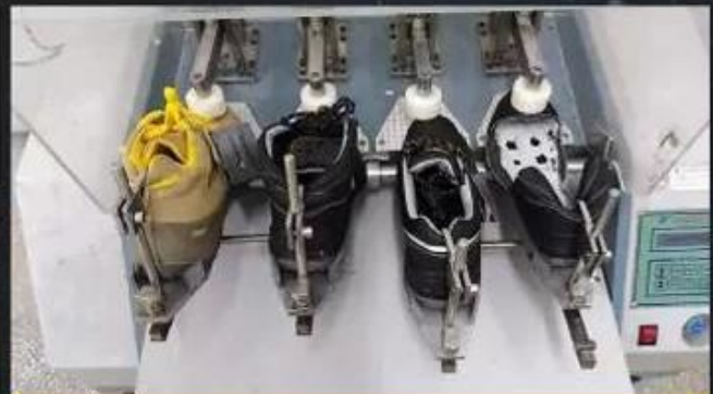
Flex Tester \geq 36,000 T
