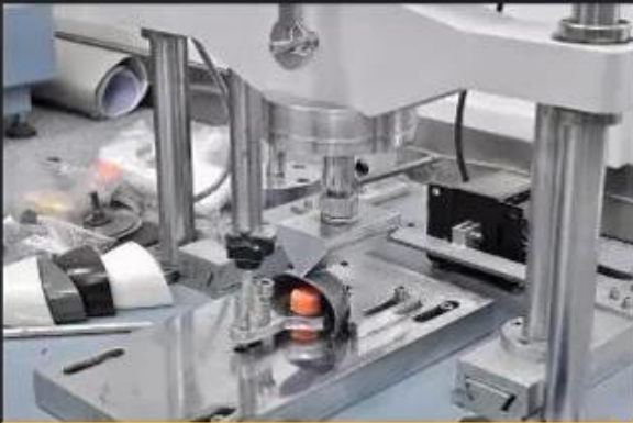
Toe cap Test \geq 200 Joules
