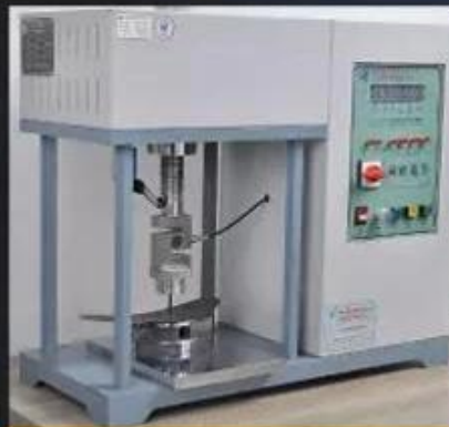
Midsole Test \geq 1200 Newtons
