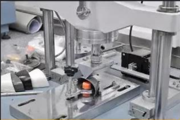
Toecap Test \geq 200 Joules
