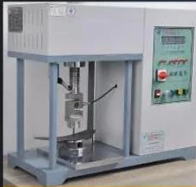
Midsole Test \geq 1200 Newtons
