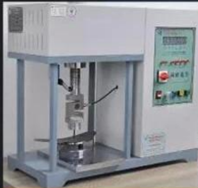
Midsole Test \geq 1200 Newtons
