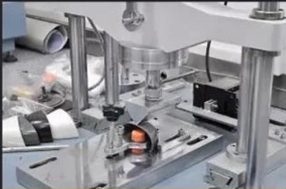
Toecap Test \geq 200 Joules
