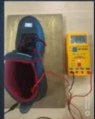
ESD Anti-Static Test
