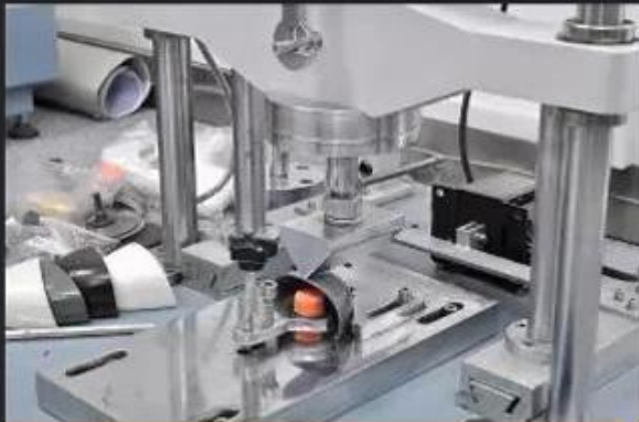
Toecap Test \geq 200 Joules
