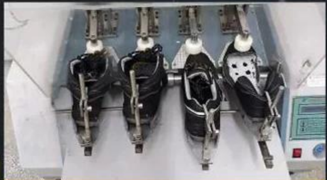
Flex Tester \geq 36,000 T
