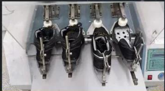
Flex Tester \geq 36,000 T
