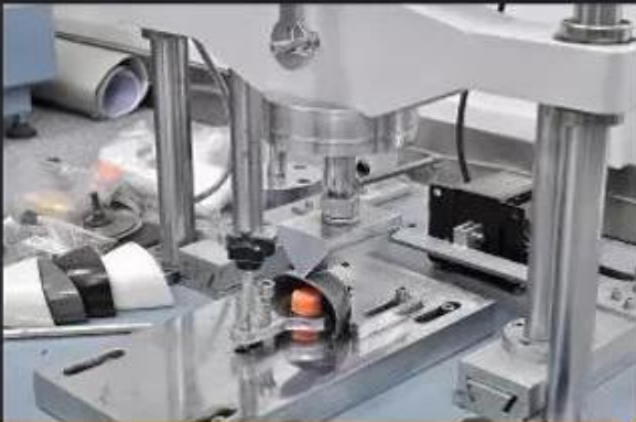
Toecap Test \geq 200 Joules
