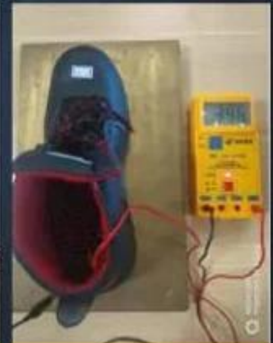
ESD Anti-Static Test
