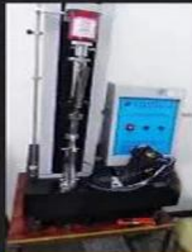
Bondness Test \geq 4.0 N/mm
