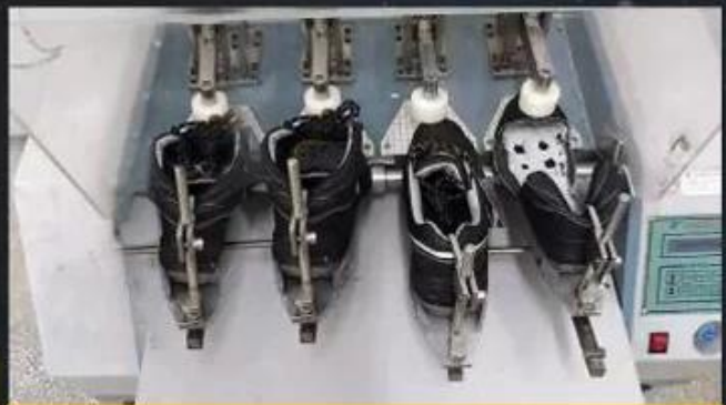
Flex Tester \geq 36,000 T
