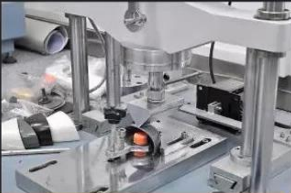
Toecap Test \geq 200 Joules
