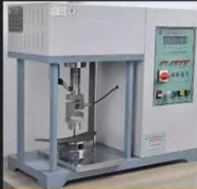
Midsole Test \geq 1200 Newtons
