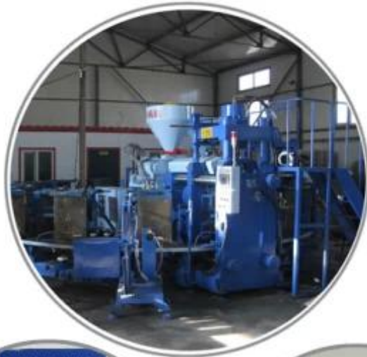
Automatic Injection Molding Machine
