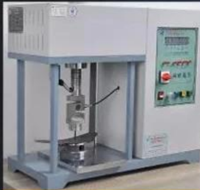
Midsole Test \geq 1200 Newtons
