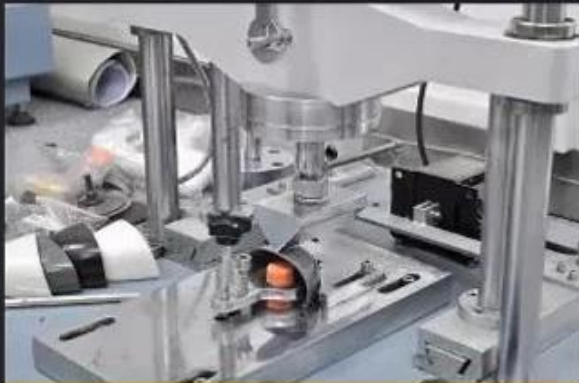
Toecap Test \geq 200 Joules
