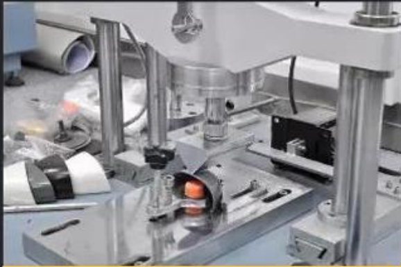
Toecap Test \geq 200 Joules
