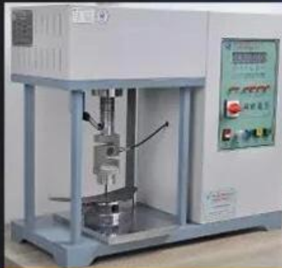
Midsole Test \geq 1200 Newtons
