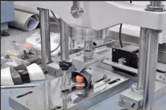
Toecap Test \geq 200 Joules
