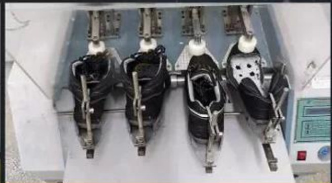
Flex Tester \geq 36,000 T
