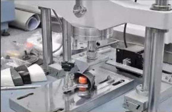
**Toecap Test  $\geq 200$  Joules**
