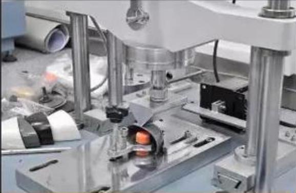
**Toecap Test  $\geq 200$  Joules**
