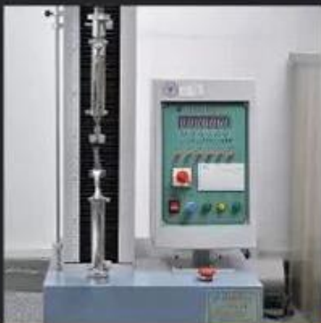
Tear Strength \geq 120 N
