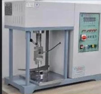
**Midsole Test  $\geq 1200$  Newtons**
