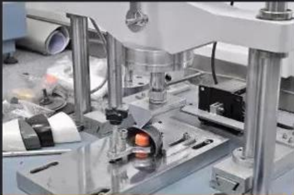
Toecap Test \geq 200 Joules
