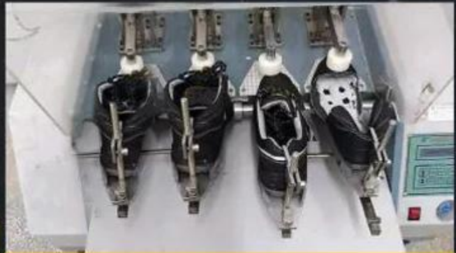
Flex Tester \geq 36,000 T
