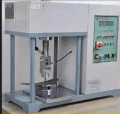
Midsole Test \geq 1200 Newtons
