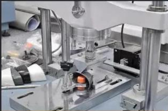
Toecap Test \geq 200 Joules
