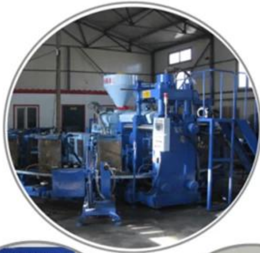
Automatic Injection Molding Machine
