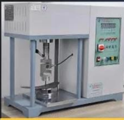
Midsole Test \geq 1200 Newtons
