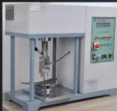
Midsole Test \geq 1200 Newtons
