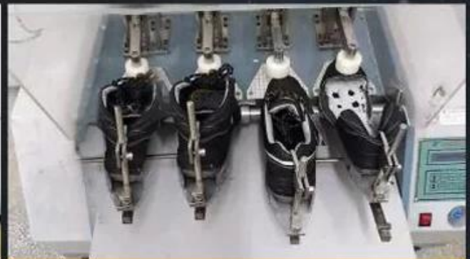
Flex Tester \geq 36,000T
