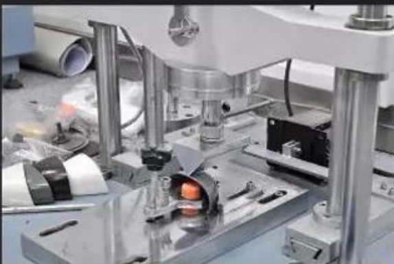
Toecap Test \geq 200 Joules
