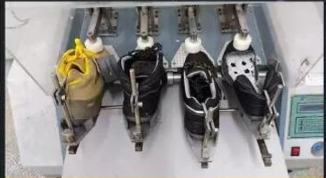
Flex Tester \geq 36,000 T
