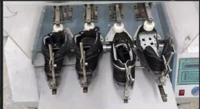
Flex Tester \geq 36,000 T
