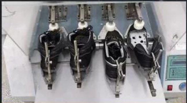
Flex Tester \geq 36,000T
